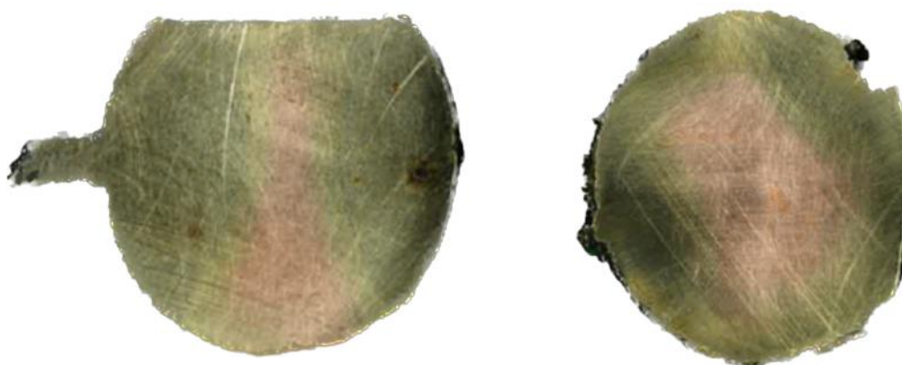
Figure 9. Cross-section reacted Cu-cylinders after approx. 1100 days in operation.
